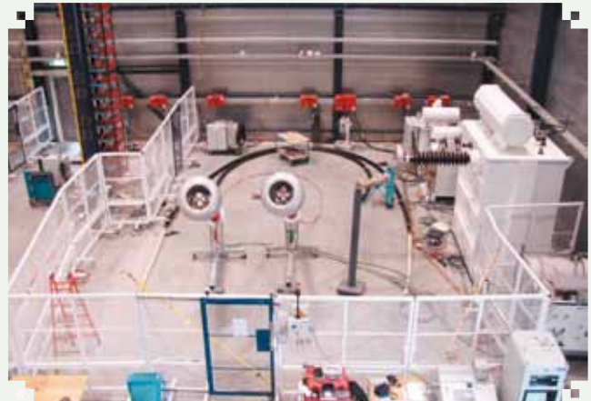
Oman Cables product samples undergoing breakdown testing in the KEMA High Voltage Test Laboratory in Arnhem, The Netherlands
